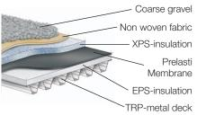
On some parts of the roof parking decks has been installed. The rubber membrane provides excellent properties for this construction due to the viscous and elastic properties that makes the material resistant to very large ballast weight.
