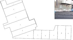
The 4800 sqm large irregular shaped concrete deck between the seven floor high apartment buildings was covered with 11 pcs of Prelasti panels tailormade to the size of the deck.
