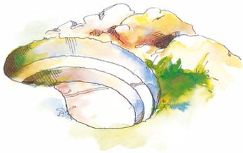
**1.** Sharp stones and roots should be removed, and a layer of sand laid on the bottom bed, alternatively a 150g/sqm thick protection layer of geotextile. To achieve varied vegetation, you can make a 25 cm deep recess all the way around.
