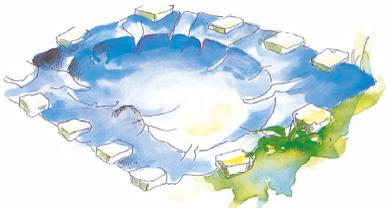
**2.** Check that there are no sharp stones or roots in the pit. Put a layer of sand or a geotextile in the bottom. Lay out the panel over the pond and place a few stones on the edges to hold the panel in place. Fill with water.
