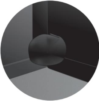
**5.** When the V-shaped part is joined, it shall then be folded and heat-welded towards one side of the inner corner.
