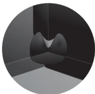
**3.** Cut a circular piece of RubberShell. Remove the release film, leaving about a third of the surface still covered by the film. Heat-weld the circular piece into the bottom inner corner.
