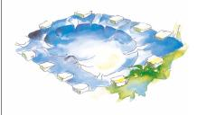
**2.** Check that there are no sharp stones or roots in the pit. Put a layer of sand or a geotextile in the bottom. Lay out the panel over the pond and place a few stones on the edges to hold the panel in place. Fill with water.
